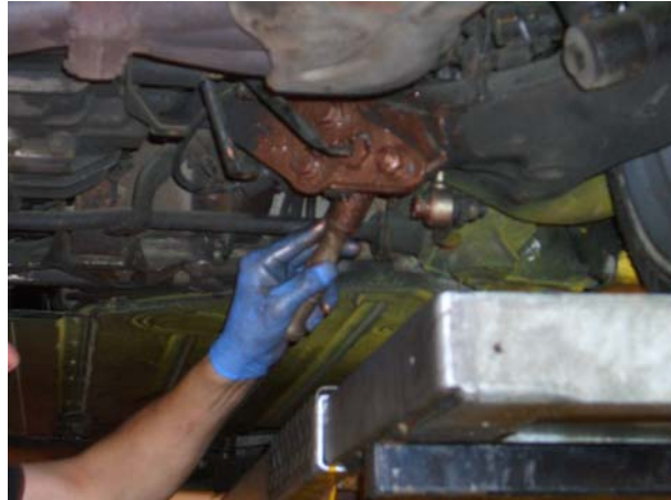
Protecting the newly adjusted parts with copper grease
